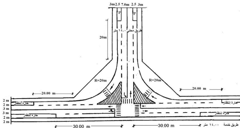
Figure 3 A proposed model for the intersection of two roads using islands in the canal solution to direct traffic
