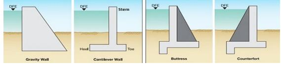
Figure 8: Types of flood walls
