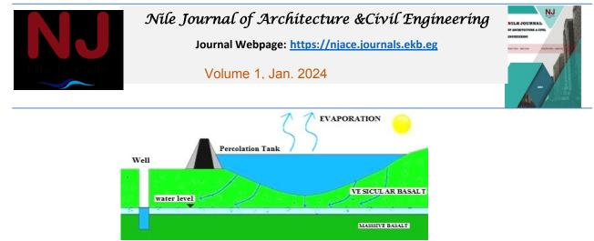
Figure 14: Rainwater Harvesting through Percolation Tank
