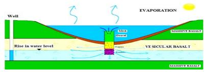
Figure 16: Rainwater Harvesting through Recharge Shaft
