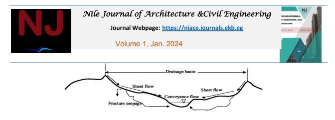
Figure 3: Sheet and channel flows
