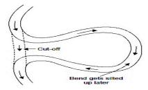
Figure 10 Cut-off in a meandering river
