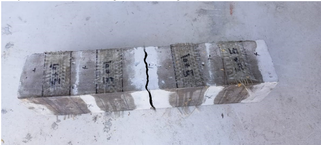
Fig. (17): Failure shape of S17
