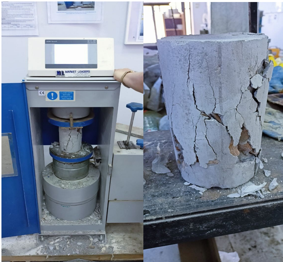
Fig. (4): Failure shape of S1
