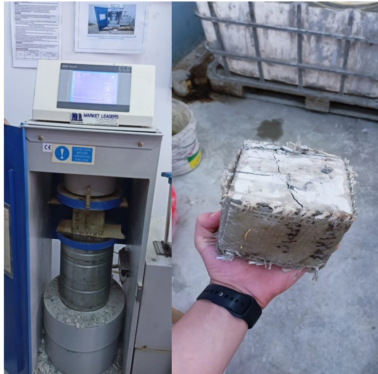
Fig. (10): Failure shape of S11.
