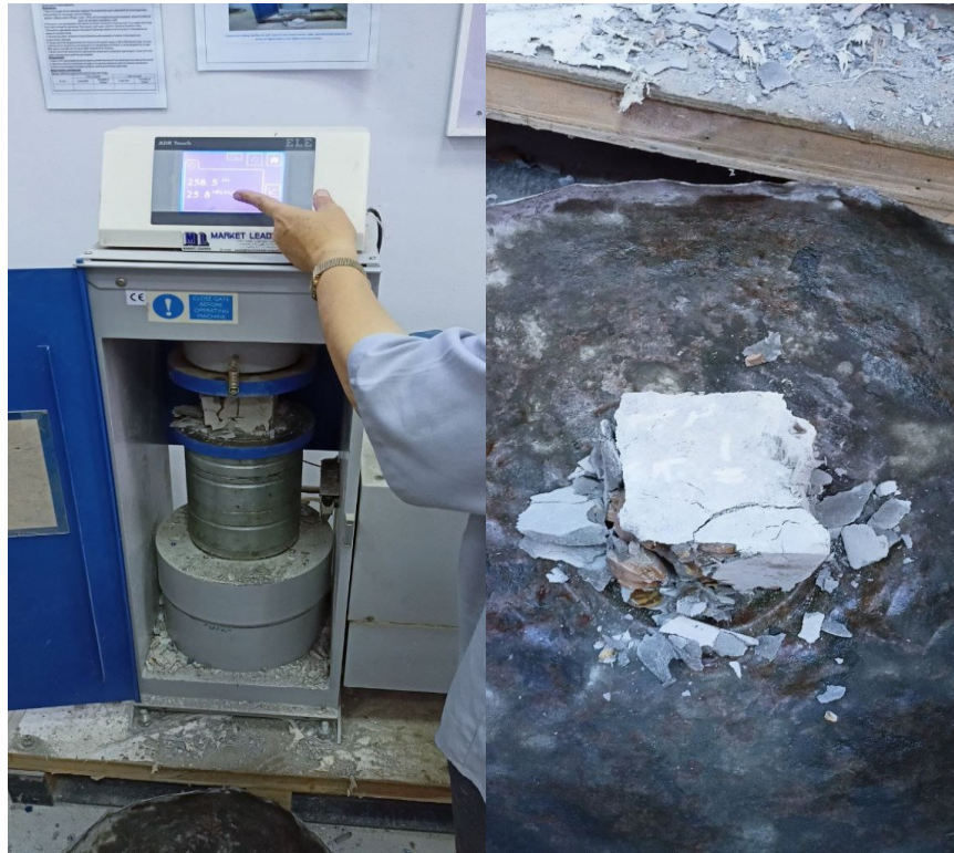
Fig. (8): Failure shape of S3&S4.
