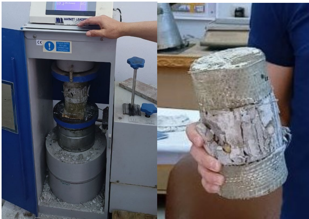
Fig. (5): Failure shape of S7
