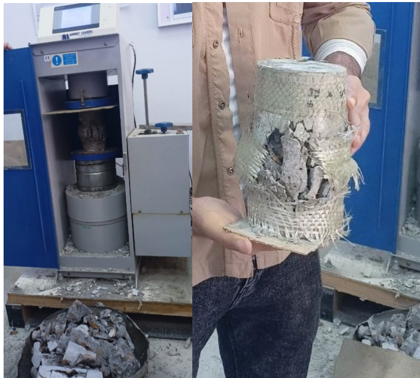
Fig. (6): Failure shape of S8.
